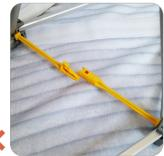
When setting up, ensure that the arms are aligned. If not, the arms will snap when pressure is applied. Use your hand to guide them together. They should not be forced into locking position.
